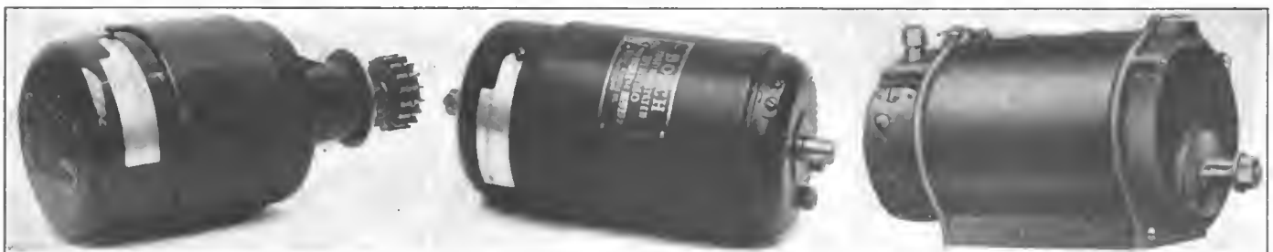
Fig. 4—Three types of Bosch lighting generators. At the left, for driving by chain. In the center, for insertion in a shaft line, for which purpose the armature shaft is carried through the casing at both ends. At the right, a special model with standard magneto base and low position of armature
